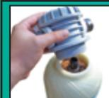
**Step A:** When output water quality has exceeded pre-determined level, or when spotting occurs, DI water is no longer being produced. Shut off water supply and remove tank head.
